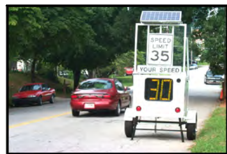
Photo 5.8: Portable variable speed display board.
