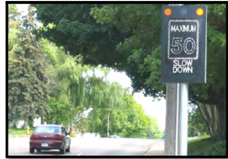
Photo 5.9: VATCS used to display warning signs to speeding drivers.
