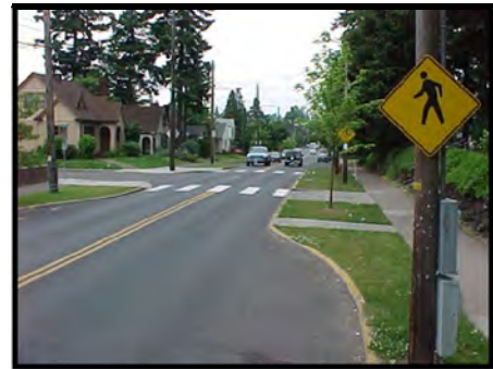
Photo 5.18: Intersection with curb bulb-outs.
